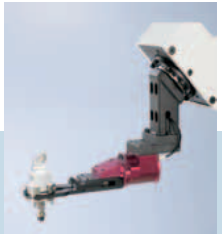
Gripper change With reference to the tooling system version, grippers are exchanged automatically.
