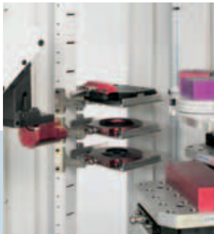
Gripper dock Grippers and covers are stored outside the workpiece magazine to save space.
