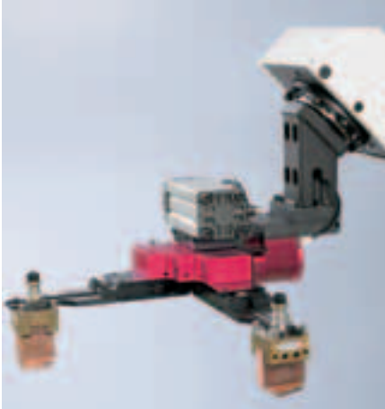
Fast workpiece change with double gripper The gripper is automatically allocated and exchanged correctly.
