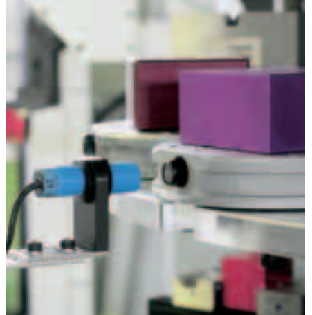
Workpiece identification within seconds EWIS™ Rapid identifies all the cell positions and transmits them to the cell computer.
