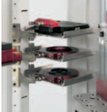
Automated covers The chucks remain protected. Operative safety is increased.
