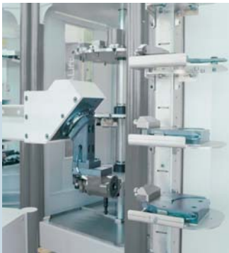
To save space, all EROWA system carriers required are stored in the gripper dock.
