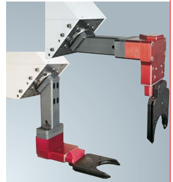
CNC machines with vertically aligned chucks can also be served by the ERS. The swivelable gripper arm turns the palletized workpiece into the correct position.
