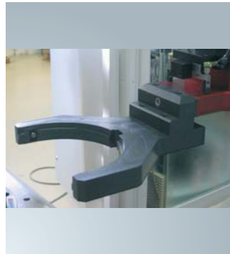
Gripper for PC210 pallets; maximum transfer weight: 100kg.
