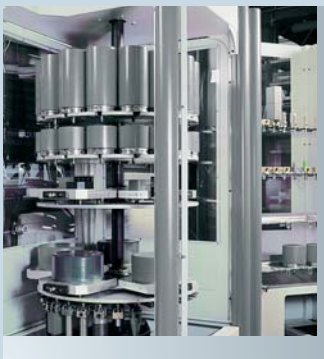
Up to 9 levels are possible. Individual combination of magazine plates. Maximum load: 1200kg.
