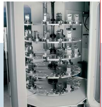
Magazine configuration for series operation. 5 levels with 15 positions each results in 75 pallet positions.
