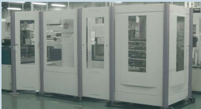
CE-conforming safety barriers are an integral part of the facility.
