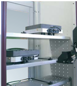
Magazine with vacuum coupling for the permanent clamping of pallets.
