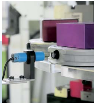
EWIS™ Rapid records all the magazine positions and communicates them to the cell computer.
