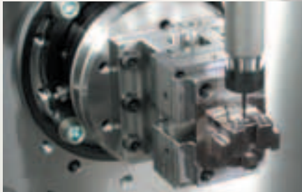
Optimally accessible for horizontal and front-side machining.
