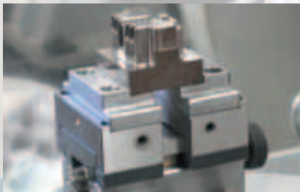
Stable clamping with minimum clamping depth.
